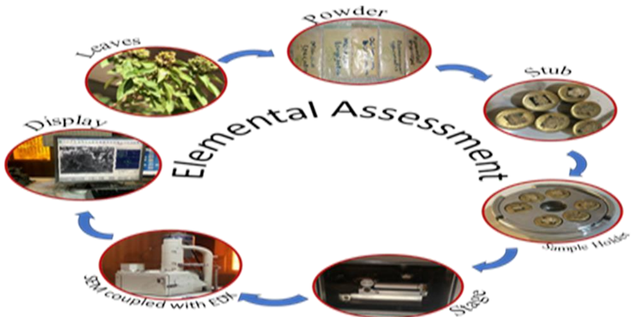
Figure 6. Different steps of elemental analysis
