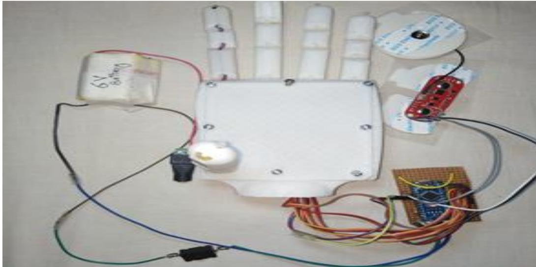
Figure 4. Completely assembled prosthetic hand, sensor, circuit board, and battery
